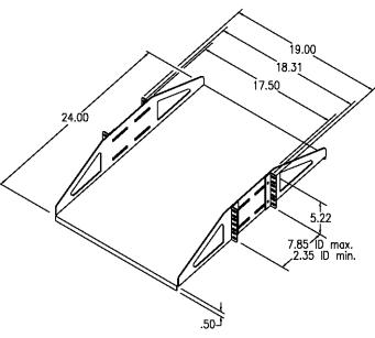
D-4460 Fixed Relay Rack Shelf is designed to fit 19" open relay racks - adjustable mounting brackets are included.
