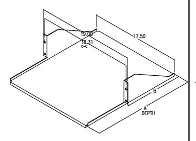
D-4458 Fixed Relay Rack Shelf is designed to fit 19" open relay racks.
