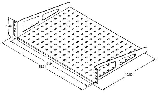
D-4456 all-in-one shelf mounts equipment on the inside or the outside of standard 19" enclosures and racks. Rugged 14-gauge steel construction.
