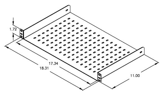
D-4455 all-in-one shelf mounts equipment on the inside or the outside of standard 19" enclosures and racks. Rugged 14-gauge steel construction.
